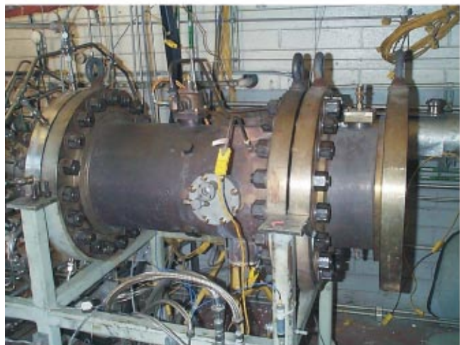
Fig. 5 Top panel: single-injector atmospheric pressure test facility at PCI. bottom panel: single-injector high-pressure test facility at Solar Turbine.
