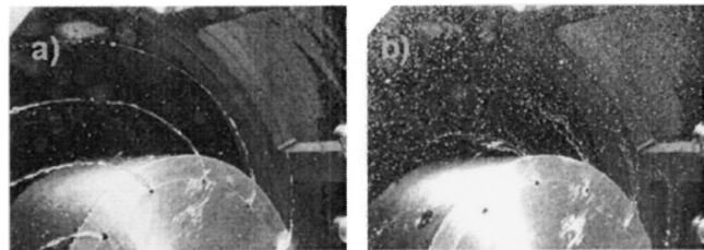
Fig. 3 Full-access visualization of axial jet disintegration. (a) \omega = 105 rad/s, q = 1.67 \cdot 10^{-5} m 3 /s, \nu_L = 5 \cdot 10^{-6} m 2 /s. (b) \omega = 524 rad/s, q = 1.67 \cdot 10^{-5} m 3 /s, \nu_L = 5 \cdot 10^{-6} m 2 /s.
