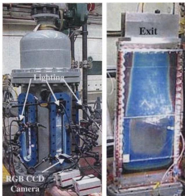
Fig. 4 Test rig pressure vessel (left) and internal test section (right, jets inactive)
